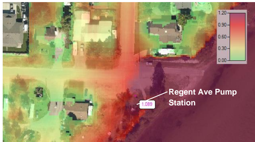
Figure 3-13: 1/200-year flood maximum depths, coloured by water threshold stages (m)
