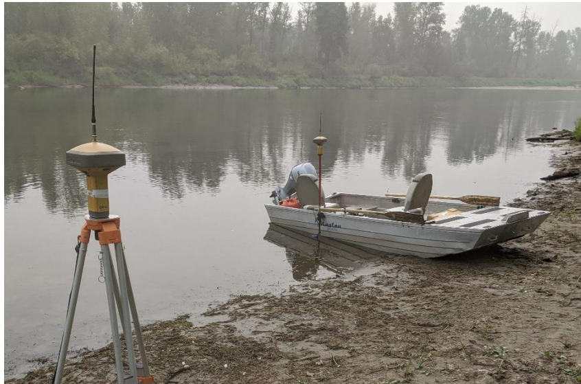
Figure 2-4: GR5 base station in foreground with GR5 rover and Lowrance Sonar set up in background, attached to boat.
